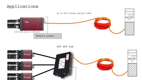
The total video bandwidth of the latter configuration is limited to 32 MByte/s due to the fact that the bus switches to 1394a speed.
