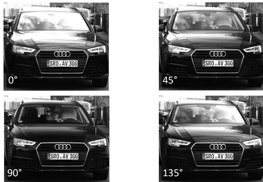
Figure 5: Polarization angle versus image brightness in sub-images
