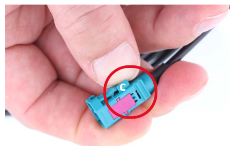
Figure 14: Pressing down the latch (c) of the HSD STP connector
