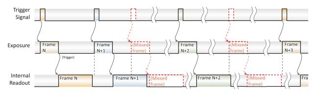
*Figure 7: Trigger timing when IntegrationMode is set to IntegrateThenRead - the overtriggering events are marked in red*
