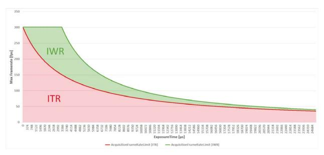
Figure 8: Maximum framerate ITR and IWR (Goldeye G-033, Mono mode: Mono8, ROI: 640x512.
