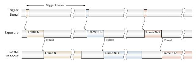
Figure 3: Trigger timing in ITR mode (rising edge trigger displayed)
