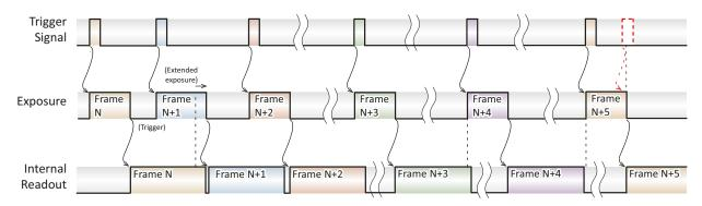
*Figure 6: Trigger timing when IntegrationMode is set to IntegrateWhileRead - varying trigger intervals, the red dashed lines mark the overtriggering event*
