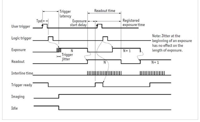
Figure 1: Trigger timing diagram
