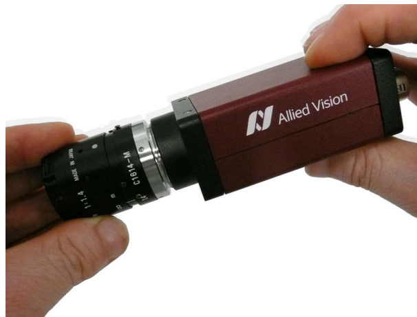
Figure 144: Illustration of camera orientation when removing lens or dust cap
