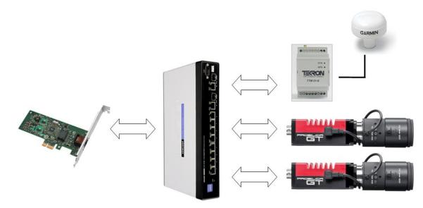
Allied Vision cameras can be synchronized to a GPS timer, allowing "real world time" synchronization. Configure PtpMode on all of the cameras to Slave or Auto. In Auto, the IEEE1588 best master clock algorithm will elect the GPS clock as the master. Each camera will synchronize to the GPS master clock.
