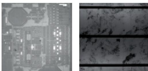
At wavelengths above 1100 nm silicon becomes transparent. Thus, SWIR cameras are perfect for analyzing metallization and electrical contact errors on the backside of wafers.
