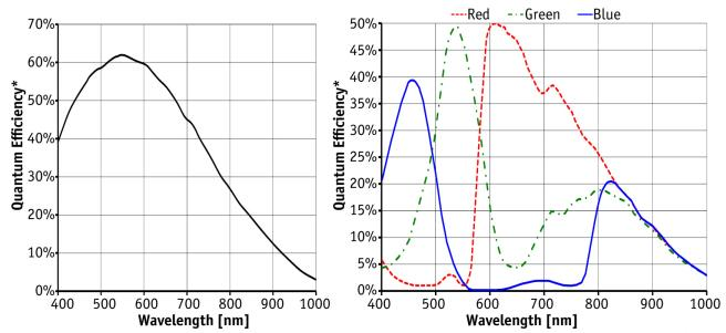
\*QE measured without protection glass or filters. With glass or filters, quantum efficiency decreases by approximately 10%.
