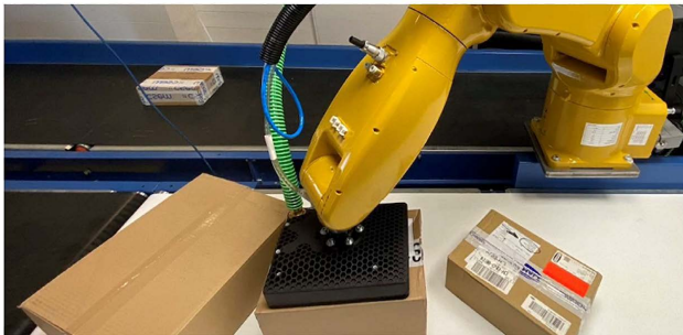
eSorter induction system: A robot isolates parcels from an incoming conveyor.
